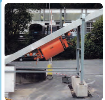
Rollover bucket in a 32° inclination = 60%
