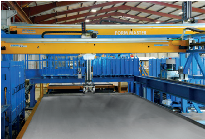
The shuttering and deshuttering robot plays a key role in the increase in efficiency and quality: the Form Master carries out all the work steps fully automatically and with high precision.
